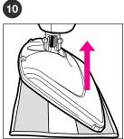
When unit has cooled, remove Ultra-Microfiber pad and empty the water tank. Store unit upright in a dry area.
